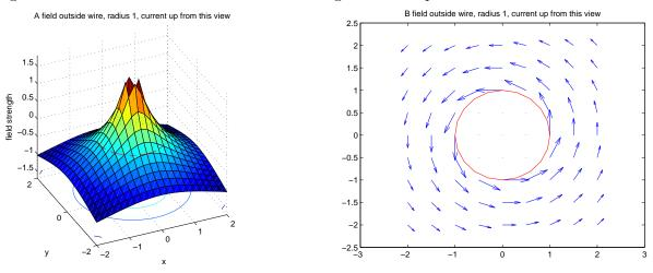
Next extend this to a single loop of wire with programs loopSection2Aplot and loopSection2Bplot. Note that the fields are additive: just add the two scalar results for A or the two vector results for  $\vec{B}$ . (In 2D A is scalar.)
