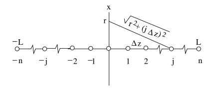
We'll suppose the charge at position j is  $Q_j$  and we'll consider all charges to be equal:  $Q_j = Q_0, j = -n : n$ . The distance from position j to (r, 0, 0) is  $r_j = \sqrt{r^2 + (j\Delta z)^2}$ . So the potential energy of a test charge q at (r, 0, 0) is
