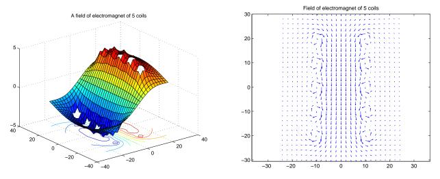
This last ("coil") is called a "solenoid". Notice that the  $\vec{B}$  field almost disappears outside the solenoid but is very strong inside.
