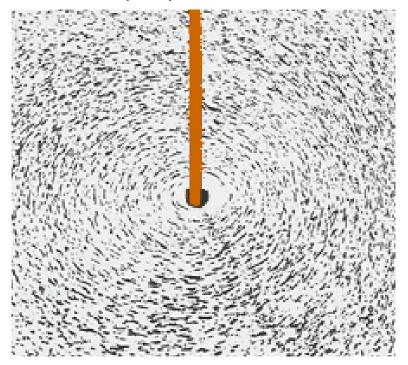
We can see the circular alignment of the filings around the wire. These circles are modelled by the curl in  $\vec{B} = \vec{\nabla} \times \vec{A}$ . Of course, curl goes too far and insists on a *direction* which we do not observe. This handedness is cancelled by a second operation to determine the force on a moving test charge—it involves a cross product
