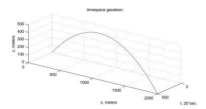
Unfortunately, to make MATLAB show the time axis on a scale comparable to the x and z axes I had to multiply t by 25: what shows as 500 is actually, still, 20 sec.
