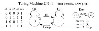
This Turing Machine [Pen89, p.41] actually adds 1 to a number, n, represented in "unary", that is, as a string of n 1s. Look up this reference and check that the state diagram and the array representation actually correspond to Penrose's notation for UN+1. Penrose also gives a Turing Machine which will double a number in unary representation, e.g., turning  $\ldots 000111000\ldots$  (3) into  $\ldots 000111111000\ldots$  (6).
