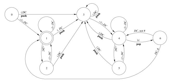
$\mathcal{DC}$  means "don't care": don't look at the stack or the input, respectively, depending on which of the two positions the  $\mathcal{DC}$  appears in.
