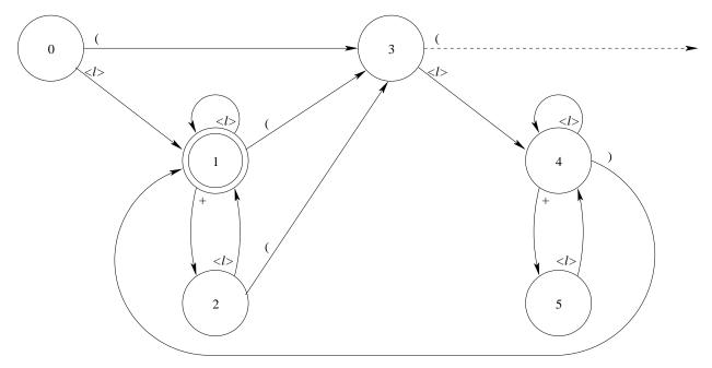
But if *nested parentheses* were allowed, e.g., (a(b+c)+d)e, then the finite automaton would fail. We'd need new extra pieces, starting at the dashed arrow transition from state 3, one piece for each allowed level of nesting.
