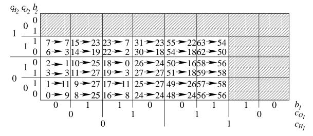
These two control systems are "on-off", or binary, and so can be modelled with boolean circuits. Even though the temperature and the comfort each have three levels, we can model them with a
