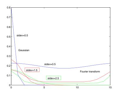
The Fourier transform of the gaussian is close to itself at stdev=1.5
