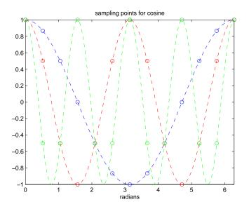
Note that the smooth cosines are plotted and that the 12 samples less than  $2\pi$  (13 including  $2\pi$ ) are highlighted with circles.
