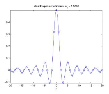
This set of coefficients goes on forever in both directions, so we must truncate to be practical. We must also shift it so that all the *n*s are non-negative, otherwise we run afoul of acausality. Doing this and running plotFilter(lowpassIdeal(pi/2,20),1) (where lowpassIdeal() is my program to calculate  $\sin(\omega_c n)/(\pi n)$  for  $\omega_c = \pi/2$  and truncated to 20 points each side of 0: you can write it for yourself) gives the following results.
