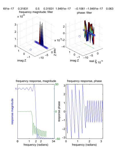
You can see how the frequency response plummets at  $\pi/2$ , halfway along the frequency range: it drops, say, 25 decibels, which means that the power drops a factor of  $10^{(25/10)} \approx 300$  (a decibel is 10 log<sub>10</sub>(power ratio)). Getting rid of the wiggles top and bottom is what you'll learn in an engineering course—except that it can never completely be done because of that truncating we did.
