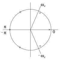
Write a program [zeroes poles] = lowpassAdhoc(wC,wNo,zeroRad,poleRad) so that lowpassAdhoc(1.22,6,1,.95) corresponds to the picture. Running plotFilter(zeroes,poles) after [zeroes poles] = lowpassAdhoc(pi/2,24,1,.95) will give the following, not so good, result.
