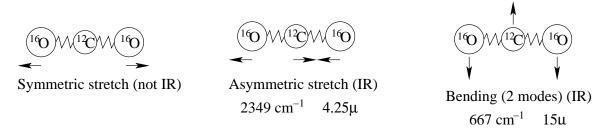
(The bending modes can be in two directions, up-and-down as shown, or back-and-forth, by rotating the whole molecule around its axis.)
