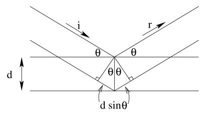
So the condition for constructive interference is  $2d\sin\theta=n\lambda$  for any integer multiple, n, of the wavelength,  $\lambda$ .
