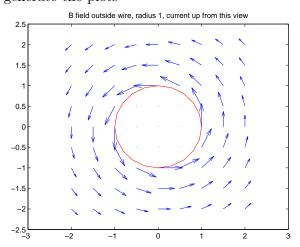
Next extend this to a single loop of wire with programs loopSection2Aplot and loopSection2Bplot. Note that the fields are additive: just add the two scalar results for A or the two vector results for  $\vec{B}$ . (In 2D A is scalar.)
