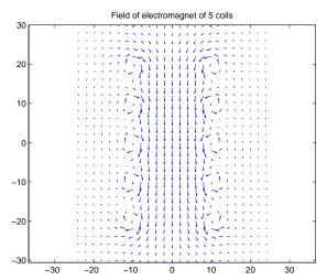
This last ("coil") is called a "solenoid". Notice that the  $\vec{B}$  field almost disappears outside the solenoid but is very strong inside.
