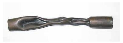
This was a nice copper tube until a bolt of lightning passed through it in New South Wales in 1905: the currents within the tube attracted each other, collapsing the tube in on itself. (And if you hear of "Z-pinch fusion", this is the sort of effect being exploited to extract fusion energy from a plasma.)
