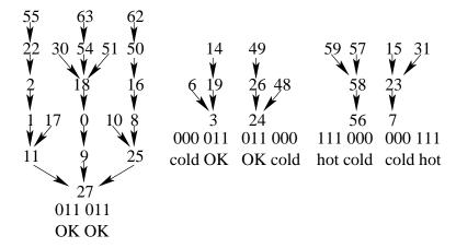
Note that this contains examples of *positive feedback* leading to *instability*: if our model did not limit the temperature to three values, one spouse could get colder and colder and the other hotter and hotter.
