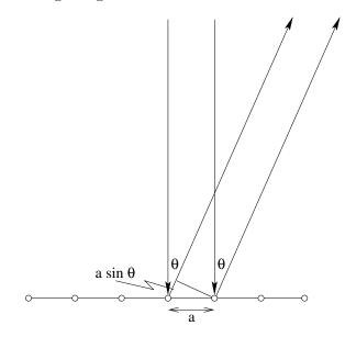
The diffraction grating has a much stronger effect than the two-slit experiment because there are many more than two ridges in the grating.
