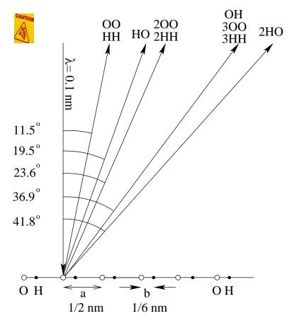
Since this atomic spacing is far too fine for visible light, so let's think about shining X-rays on it at  $\lambda = 0.1$ nm. There will be diffraction from the OO and HH spacing, a = 1/2nm, from the HO
