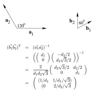
so  $b_1 = \frac{1}{d_1} \begin{pmatrix} 1 \\ 1/\sqrt{3} \end{pmatrix}$  and  $b_2 = \frac{1}{d_2} \begin{pmatrix} 0 \\ 2/\sqrt{3} \end{pmatrix}$ .
