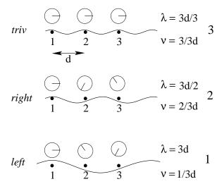
Also shown for each wave are the wavelength,  $\lambda$ , in terms of 3d, the width of the crystal (atoms spaced d apart), and the wavenumber,  $\nu$ , in terms of "per 3d". Since the wavenumber is proportional to the frequency and is just an integer in units of 1/3d, we emphasize  $\nu$  here and now on.
