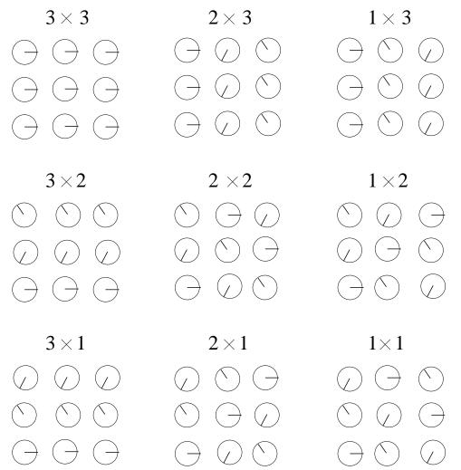
Here are plausible mode vectors, using 1 to stand for 1,  $\setminus$  to stand for  $e^{2\pi i/3}$  (the drawings above and below show why) and / to stand for  $e^{-2\pi i/3}$ .
