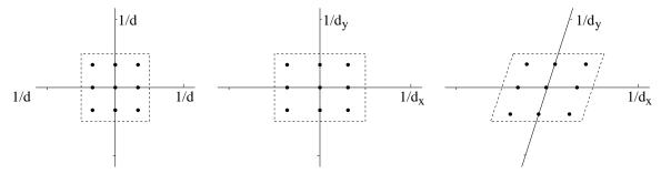
It is not hard to see that a 4-by-4 crystal would have 16 allowed wavenumbers within the same  $-[1/2d_x, 1/2d_y] \times [-1/2d_x, 1/2d_y]$  region, a 4-by-3 would have 12, and so on. So a realistically large crystal of, say  $10^{10}$ -by- $10^{10}$  atoms would have  $10^{20}$  allowed wavenumbers within the same region. There are also reciprocal lattices and Brillouin zones in three dimensions. A realistically-sized crystal might be  $10^7$ -by- $10^7$ -by- $10^7$ .
