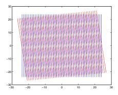
(The moiré pattern here shows clearly the irregularities in gplot, the MATLAB function I used to draw the figures.)
