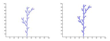
MATLAB can implement this, although in a limited way. Using quiver to draw the final picture, we can build up the picture recursively in a way which follows the symbolic string.
