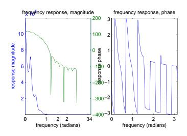
In all these discussions, an engineer must remember that there are severe constraints on the number of coefficients, due to space in the DSP chip and because of running time for the filter. So the 41 coefficients in (f) and the 24 in (g) are quite impractical.
