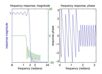
You can see how the frequency response plummets at  $\pi/2$ , halfway along the frequency range: it drops, say, 25 decibels, which means that the power drops a factor of  $10^{(25/10)} \approx 300$  (a decibel is  $10 \log_{10}(\text{power ratio})$ ). Getting rid of the wiggles top and bottom is what you'll learn in an engineering course—except that it can never completely be done because of that truncating we did.
