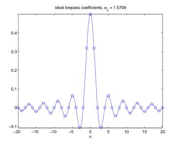
This set of coefficients goes on forever in both directions, so we must truncate to be practical. We must also shift it so that all the ns are non-negative, otherwise we run afoul of acausality. Doing this and running plotFilter(lowpassIdeal(pi/2,20),1) (where lowpassIdeal() is my program to calculate  $\sin(\omega_c n)/(\pi n)$  for  $\omega_c = \pi/2$  and truncated to 20 points each side of 0: you can write it for yourself) gives the following results.
