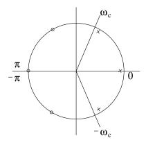
Write a program [zeroes poles] = lowpassAdhoc(wC,wNo,zeroRad,poleRad) so that lowpassAdhoc(1.22,6,1,.95) corresponds to the picture.
