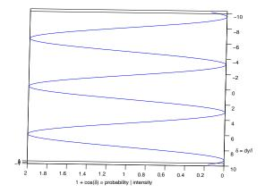
So if we know how far apart the bright spots are on the screen  $(\Delta y)$ , and also d and L, then we can find  $\lambda$ , the wavelength of the light.
