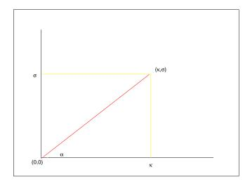
3. A horizontal polarizing filter extracts the  $\kappa$  component.
