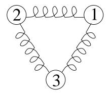
This system must be described as a combination of the three-element permutation of the three atoms (the **perm** representation) and the 2-D motions of each atom  $(x_1, y_1), (x_2, y_2), (x_3, y_3)$  (the **2D** representation).
