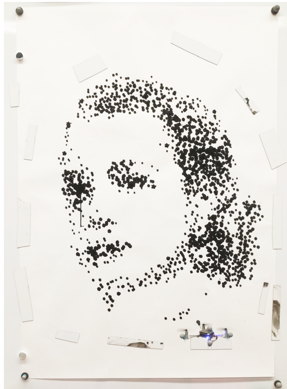
Fig. 1. The untethered quadrotor executing a stippled print of Grace Kelly with 2000 dots. With an untethered robot, approximately 40 separate flights are required to complete the print due to battery limitations.
