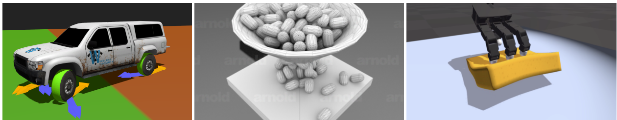
Figure 1: The Matchstick model allows for control of frictional behaviour in situations such as tire ground contact, a hopper, and soft robotic gripping, where each example shown here also uses different simulators with different contact solvers (Vortex, PROX, and Flex).
