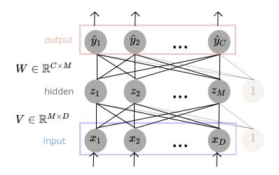
objective  $\min_{W,V} \sum_n L(y^{(n)}, f(x^{(n)}; W, V))$  loss function depends on the task
