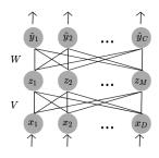
objective  $\min_{W,V} \sum_n L(y^{(n)}, f(x^{(n)}; W, V))$
