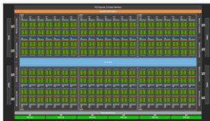
NVIDIA A100 Ampere ~54B transistors
