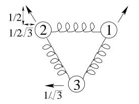
How did we get this breakdown? First we got a' by normalizing the last column of the matrix M. Think of this as disturbing the system by pulling down on atom 3, or, mathematically, by operating with M on v = (0, 0, 0, 0, 0, 1)'.
