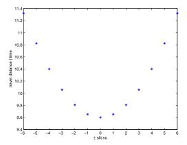
The distance travelled does not vary much for light passing through slit 0 and nearby slits. As the slits get further away from 0, the distance travelled varies (increases) much more rapidly.
