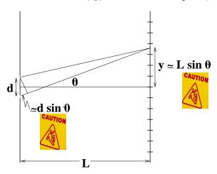
$\delta$  is the *phase difference* between the two paths, and equals what is shown as  $d\sin\theta$  in the figure, where d is the separation between the two slits.
