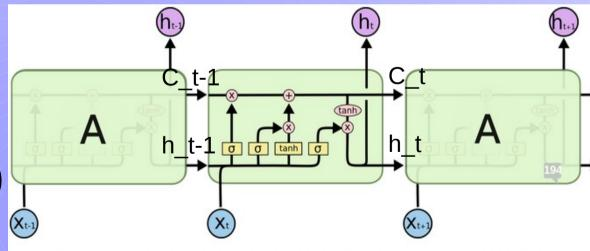
The repeating module in an LSTM contains four interacting layers. Colah's blog: http://colah.github.io/posts/2015-08-Understanding-LSTMs/
