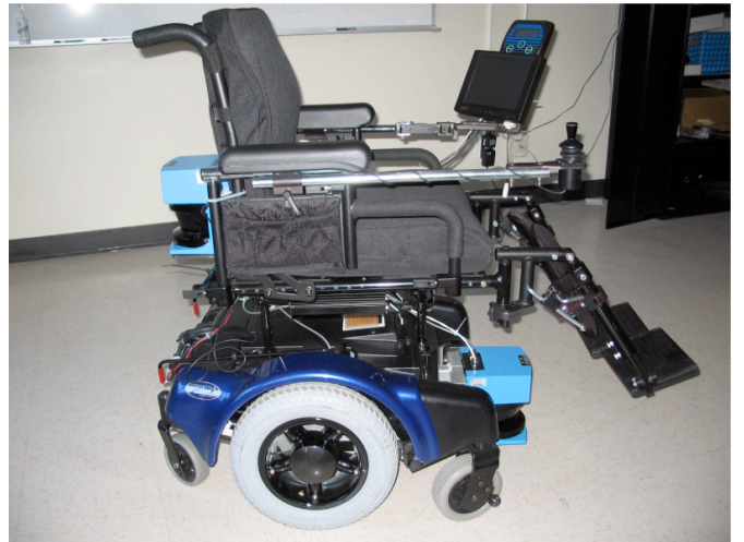
Fig. 1 The robotic wheelchair platform.
