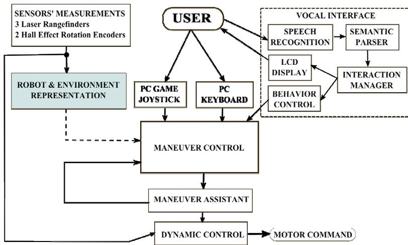
**Alternative Text Description of Figure 2: Intelligent Powered Wheelchair Architecture**
