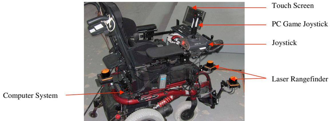
**Alternative Text Description of Figure 1: The Intelligent Powered Wheelchair Prototype Based on Quickie 646.**
