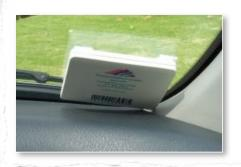
The most cost-efficient way to pay for highway use is to open an account with the 407 ETR system. Registered vehicles require a small electronic tag, called a transponder, to be attached to the windshield behind the rear-view mirror. Transponders are leased for a small monthly fee. The registration includes the owner's personal data, and vehicle details.
